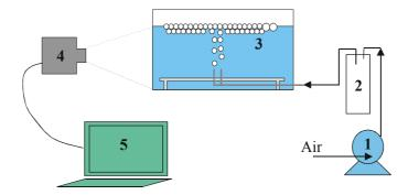
Fig. 1. Experimental set-up for CCC measurements: 1) peristaltic pomp, 2) equalizing tank, 3) cell, 4) digital camera, 5) computer
