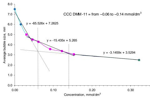
Fig. 5. Critical coalescence concentration (CCC) for DMM-11
